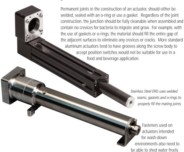
Avoid socket head bolts, counter bored holes, slotted screws or fasteners with knurling as they all have debris collection points.
